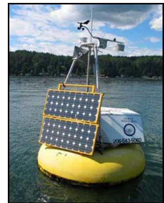
UW monitoring buoy near Belfair used to measure dissolved oxygen levels.
